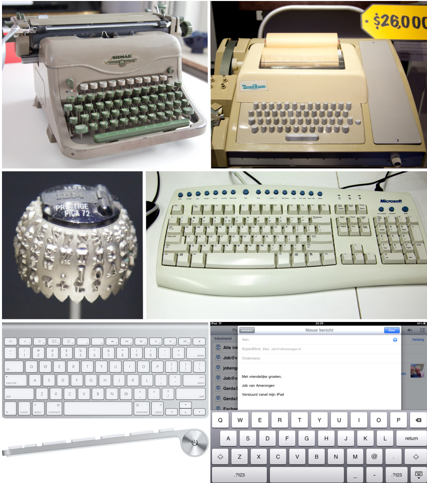
FIGURE 14 From typewriter to virtual keyboard: Top left: typewriter, top right: 'Teletype' centre left: IBM Selectric ball, centre right: PC keyboard bottom left: Apple keyboard, bottom right: virtual keyboard iPad
