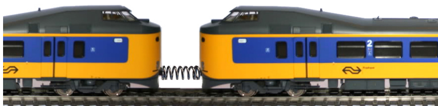
FIGURE 20 Alternative coupling mechanism: virtual spring
