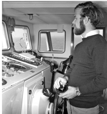
FIGURE 7 left: Autopilot, build with op-amp modules right: Adjusting the desired heading with a potentiometer
