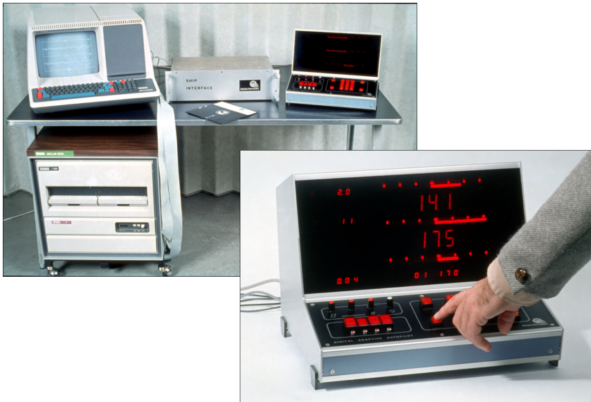
FIGURE 9 DEC LSI-11 computer with the user interface
